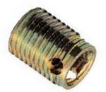
No tapping is required; just drill out the damaged threads using fractional or wire gauge drill bits. Then screw in the TufThred using a bolt and nut as an installation tool.
